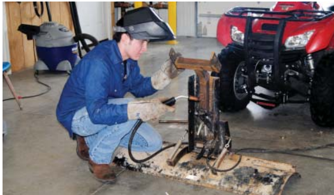
Jeremy Frazier welds together a mounting bracket to attach a snow plow to a four wheeler. Linn County R-1 Ag Class.
